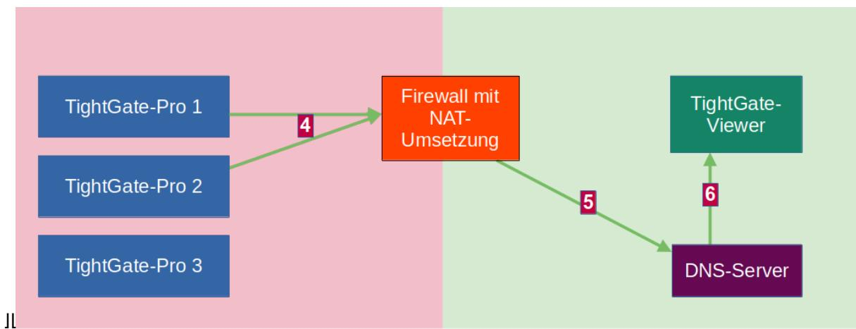
The TightGate-Pro load balancers respond in step **4** to the DNS translator which TightGate-Pro servers are currently available. In doing so, TightGate-Pro immediately returns the correct **LAN IP addresses** (in the example TightGate-Pro 1 and 3, which corresponds to the IP addresses 192.168.1.100 and 192.168.1.103). The DNS converter forwards these addresses in step **5** to the internal DNS server, which forwards them in step **6** to the TightGate-Viewer.
