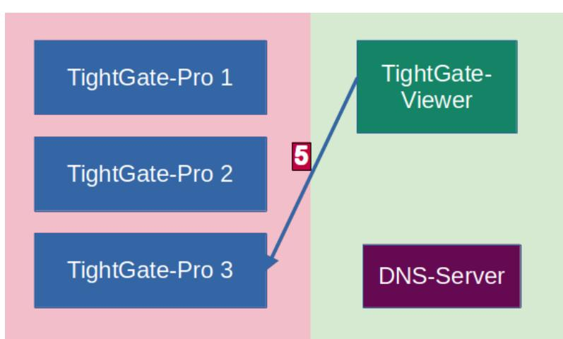
In step **5** the TightGate-Viewer makes a connection request to the IP address of the returned TightGate-Pro server.
