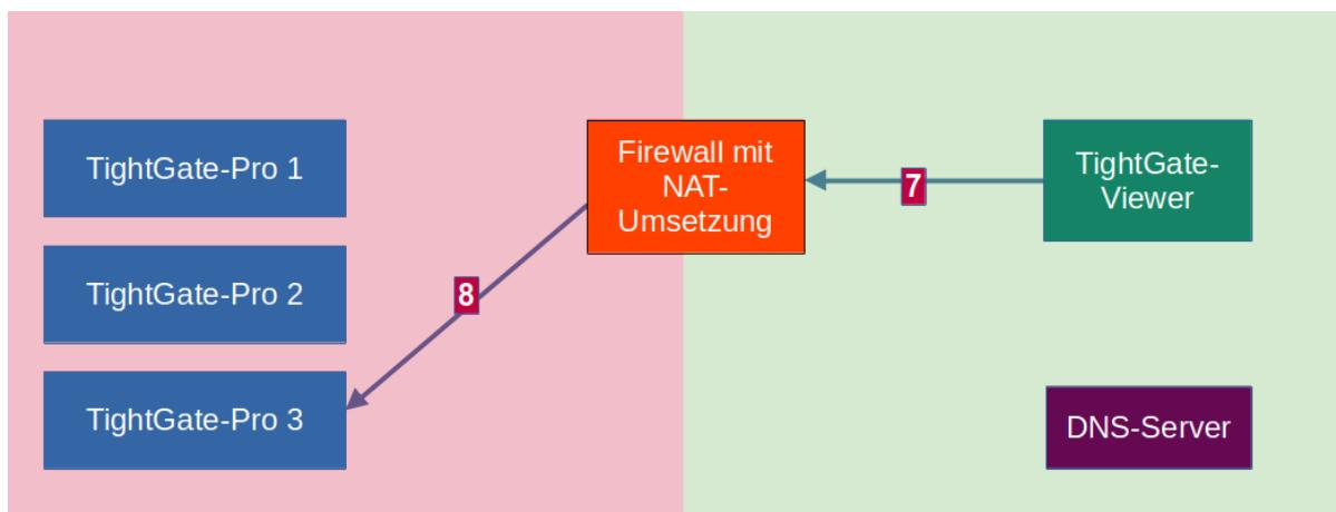
The TightGate-Viewer can now be opened in step **7** make a connection request with the correct LAN address of the available TightGate-Pro server (192.168.1.103 in the example). The NAT converter knows that the address must be NAT converted to the NAT address of TightGate-Pro 3 (10.10.10.103 in the example) and establishes the connection in step **8** establishes the connection.
