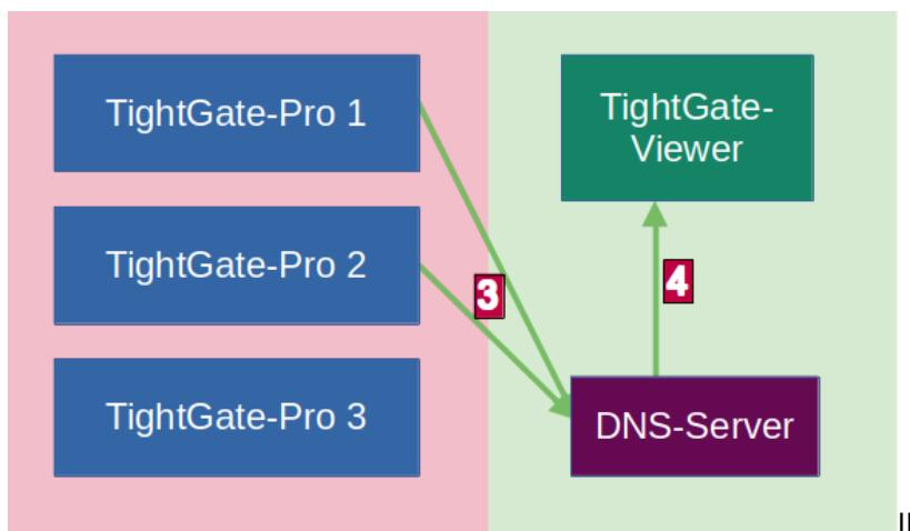
In response, the DNS server in step **3** the response from the TightGate-Pro load balancer as to which TightGate-Pro servers are available (in the example TightGate-Pro 1 and 3). From this response, the DNS server selects one (in the example TightGate-Pro 3) and returns it in step **4** to the TightGate-Viewer in step 4.
